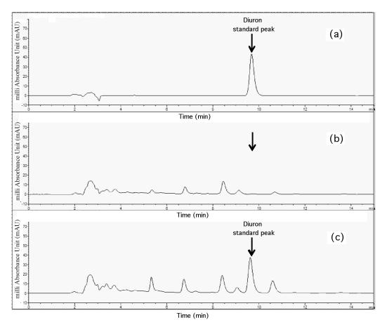
FIGURE 3. Chromatograms obtained for (a) diuron standard solution, (b) blank CPKO sample and (c) spiked CPKO sample (0.6 µg g<sup>-1</sup>)
