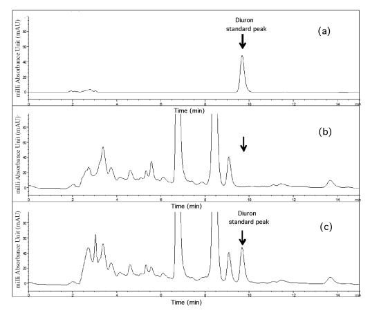
FIGURE 2. Chromatograms obtained for (a) diuron standard solution, (b) blank CPO sample and (c) spiked CPO sample (0.6  $\mu g g^{-1}$ )
